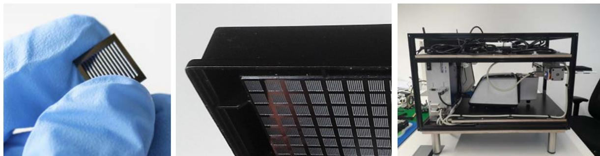
*Left: Silicon ATR crystal with v-grooves on the bottom side. Middle: Bottom side of the microplate. Right: Prototype of ATR high-throughput device.*
